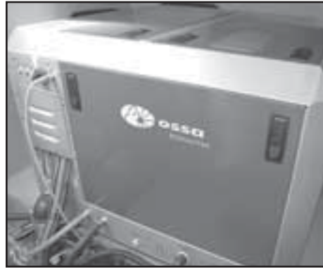
Glacier Bay Ossa Powerlite generator/engine unit.
