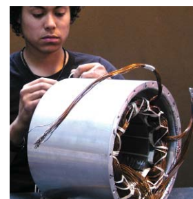
Glacier Bay generators and motors are hand wound and individually tested.
